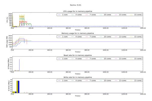
As can be seen, the execution on a single core takes a lot more time than it does on multiple cores. This has a strong effect on the efficiency as can be seen in the next plot.
