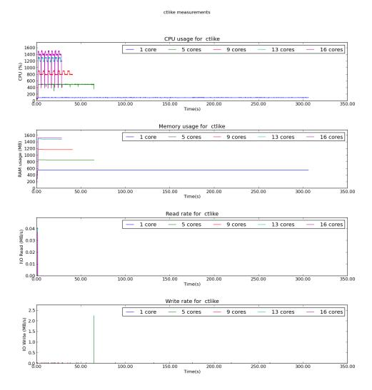
The measured speedup does not conform with the value predicted by Amdahl's Law. However, it can be seen that the execution time is greatly reduced when using multiple cores. Further investigation is needed to see why the OpenMP parallelization fails to yield an ideal efficiency.
