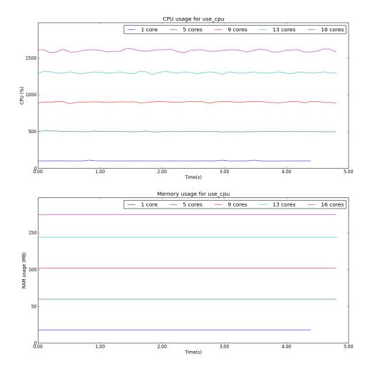
As can be seen from the plots, the CPU usage is properly monitored when there are multiple cores being employed. A somewhat strange side effect is the increase in memory as the number of cores increases.
