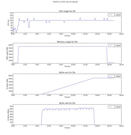
As can be seen from the plot, the cumulative write size is 5 GB and also the memory usage is about 5 GB, the extra coming from the libraries that need to be loaded. Therefore, the Monitor class and its methods yield accurate results when it comes to disk I/O.
