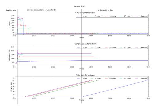
The plots show that the serial part of the program and especially the part in which I/O is done is the most time consuming one. We can therefore assume that for a process with such long serial execution time, the speedup obtained from executing the process in parallel will not scale linearly.
