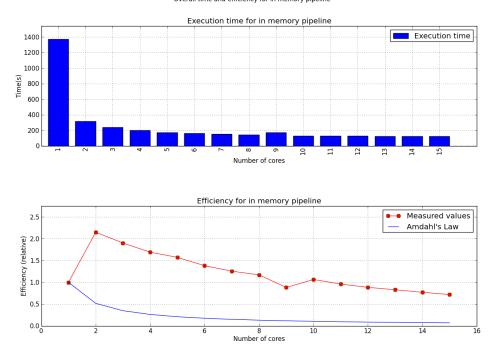
Overall time and efficiency for in memory pipeline
