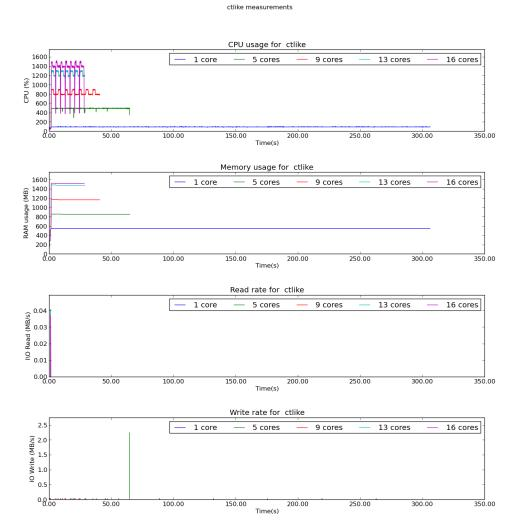
As was expected, ctlike is doing almost no I/O at all. Another important point to note is that the biggest part of ctlike is parallelized so we can expect good speedups when using multiple cores.
